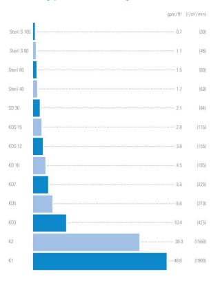
Conditions:  $\Delta$  p = 14.5 psi (100 kPa, 1 bar), Medium: Water at 68 °F (20 °C)
